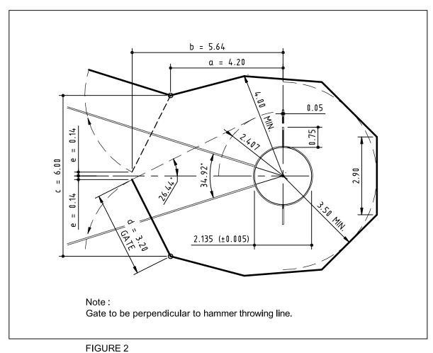
Hammer throwing cage with 3.2m gates (Dimensions in m)
